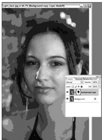
The black part in the layer mask lets the underlying image show through
